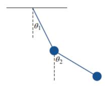
The equations describing this system depend on the angles  $\theta_1$  and  $\theta_2$ , the gravitational acceleration g, and the length L of the strings.
