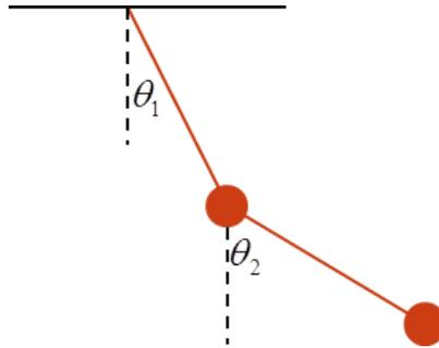
The equations describing this system depend on the angles  $\theta_1$  and  $\theta_2$ , the gravitational acceleration  $g$ , and the length  $L$  of the strings.
