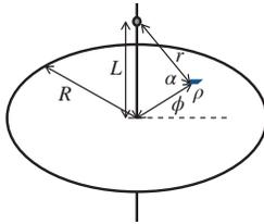
By symmetry we know the force of the disk will point straight down, so we only need to find the  $z$ -component. The force points directly along the line labeled  $r$ , so  $dF_z = -dF \sin \alpha = -dF(L/r)$ , where  $\alpha$  is the angle labeled in the picture. Putting everything together
