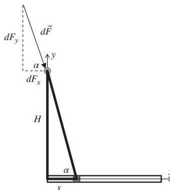
From this picture  $dF_x = dF \cos \alpha = (x/r)dF$ . The total  $x$ -component of the force of the rod on the mass is the sum of all the individual  $x$ -components:
